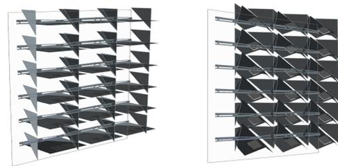
Figure 1: Cross-sectional view of the proposed FOS when fully open and fully closed, respectively.
